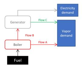
Ratio of steam production: It is used to associate a specific quantity of fuel to a unit of vapor generated in the boiler.
