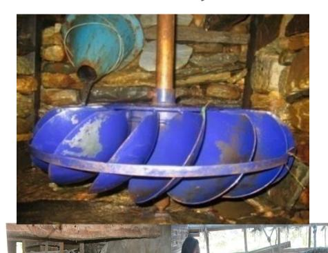
Traditional water mills is displaced by IWM. Alternately an IWM is installed by new user who might possibly have been the diesel mill entrepreneur.
