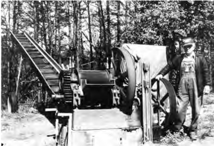
Figure 1. A typical large mill for squeezing the stalks
