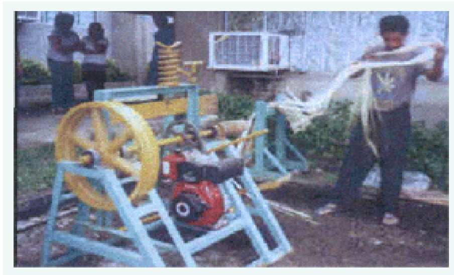
Figure 1. Portable Abaca Spindle Stripping Machine
