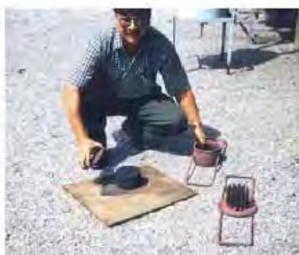
Figure 7.6: Briquette-making using the mould
