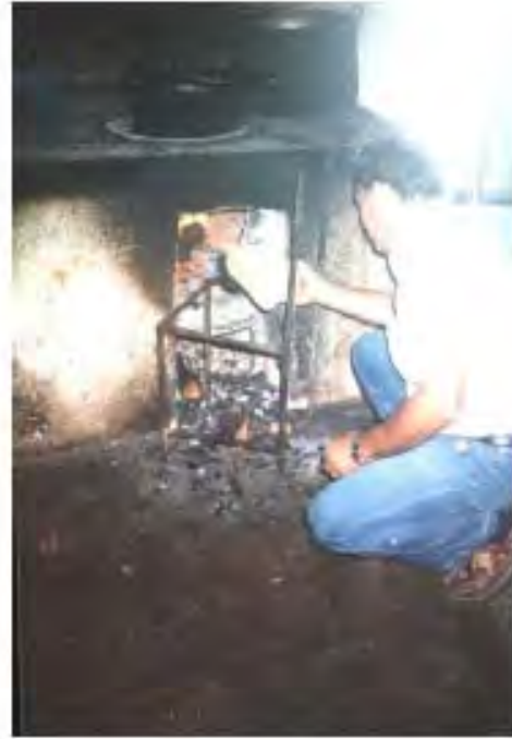
Fig. 9: SFBs feeding in the burning chamber
