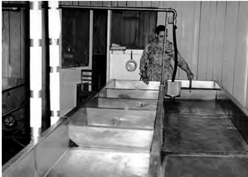
Figure 2. Evaporation Pan used for large operations
