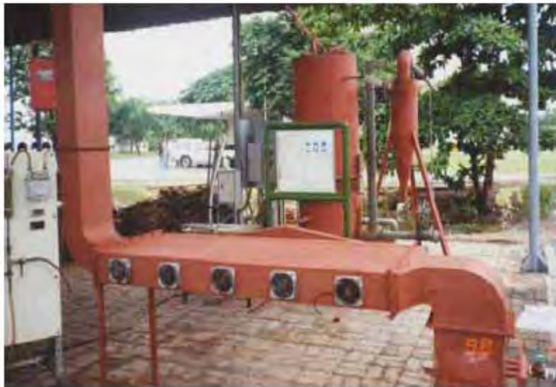
Figure 3.3: Biomass stove-heat exchanger unit without insulation
