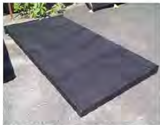
Figure 10.2: The Unglazed Transpired Solar Collector used in the Dryer
