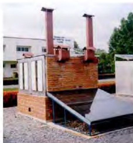
Figure 2.2 Solar-biomass hybrid cabinet dryer
