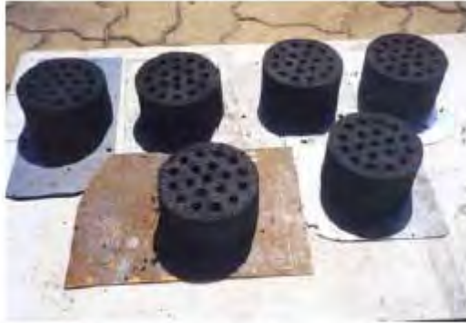
Figure 7.7: Drying of molded honeycomb briquettes
