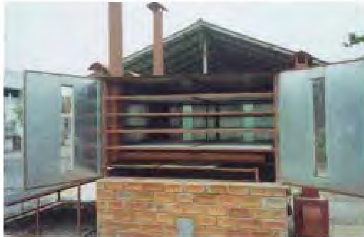
Figure 2.3: Inside view of the drying chamber
