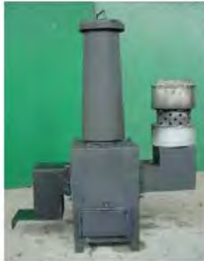
Figure 2.5: Fully assembled domestic gasifier stove
