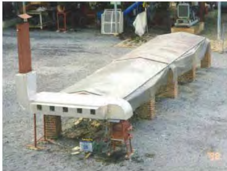
Figure 3.1: The solar-biomass hybrid tunnel dryer
