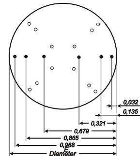
Simplified drawing of the NF.X10.112 norm, for measuring points, as per the method "Log. Tchebycheff".
