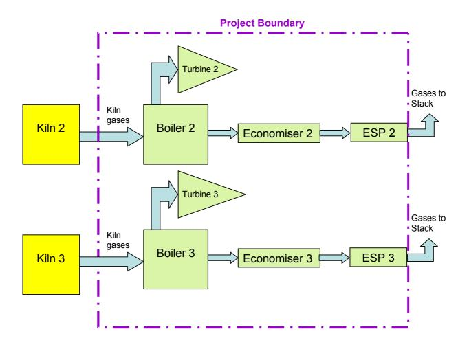
The project boundary starts from supply of waste heat at the boiler inlet to the point of electricity generated for ISL. In the absence of the project activity the same quantity of electricity would have been generated from the coal based thermal power plant. The coal based electricity generation is having higher emissions
