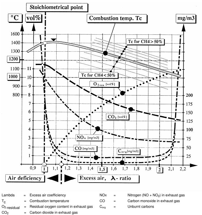
From this, it is clear that the minimum emission of contaminants is given in the combustion range of Lambda = 1,5...2.
