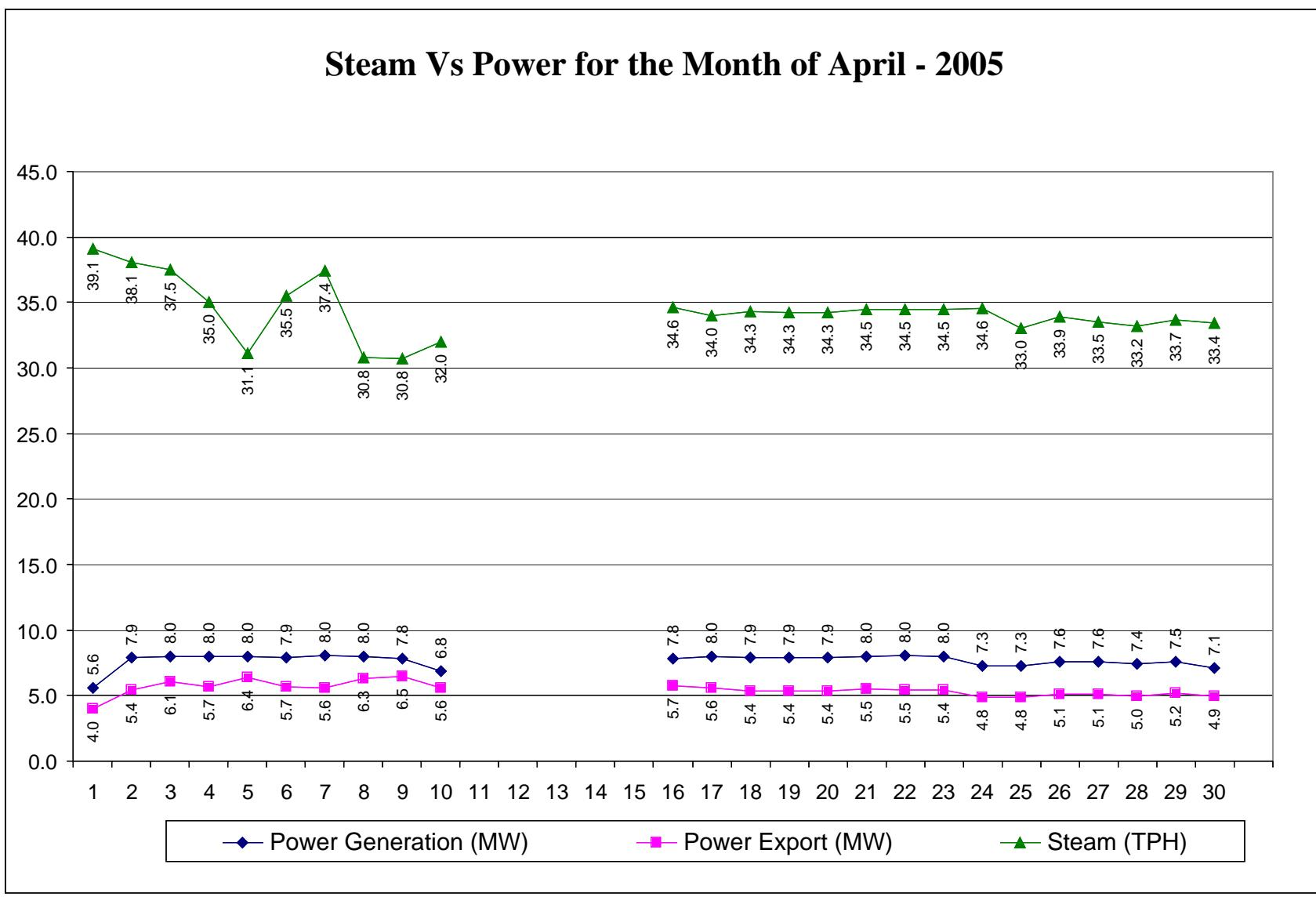
1. STG stopped on 10.04.05 and synchronised on 16.04.05 at 11.15 A.M
