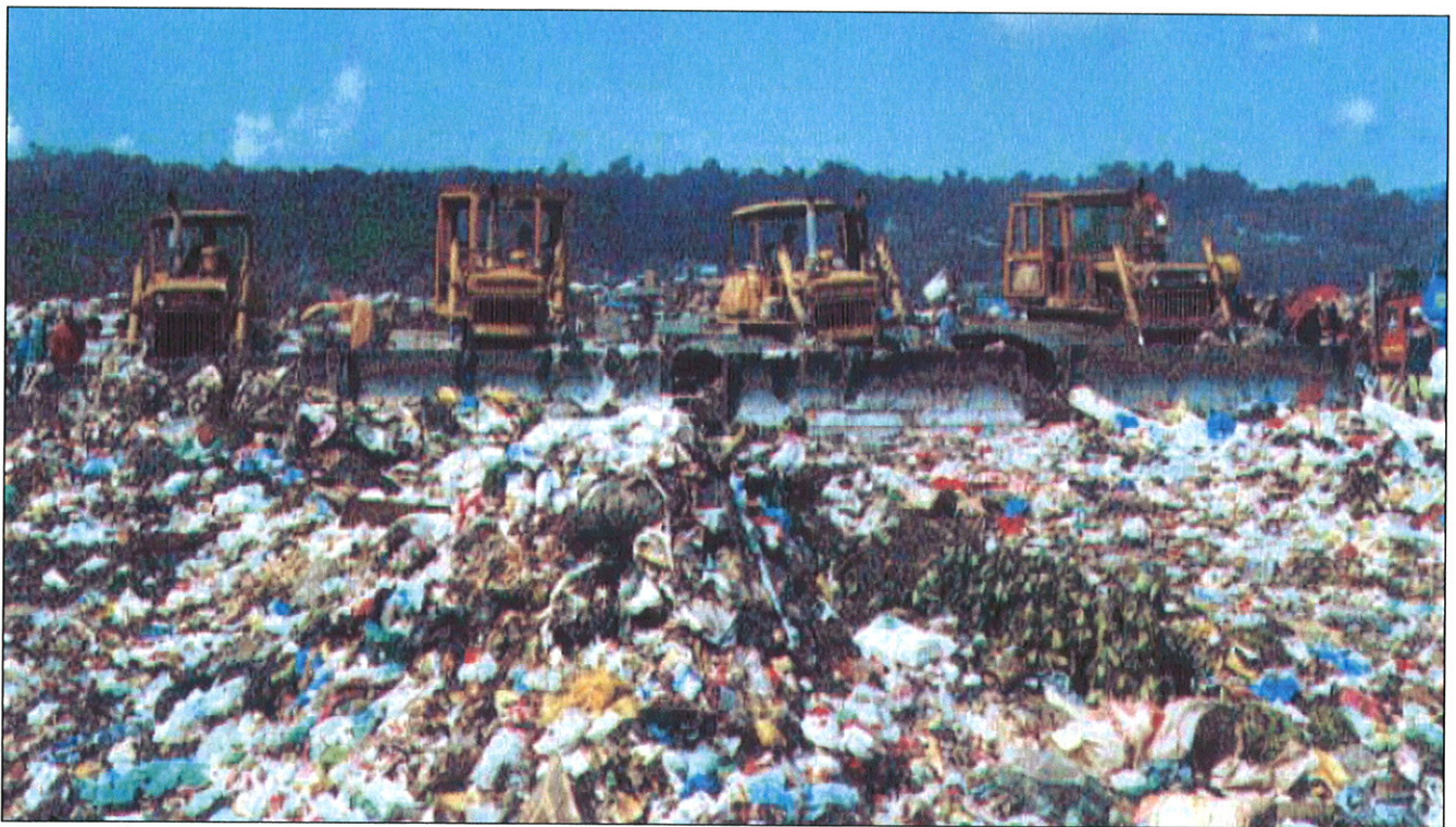
Figure 5 – Payatas landfill waste disposal operation: pushing and leveling of the wastes by bulldozer
