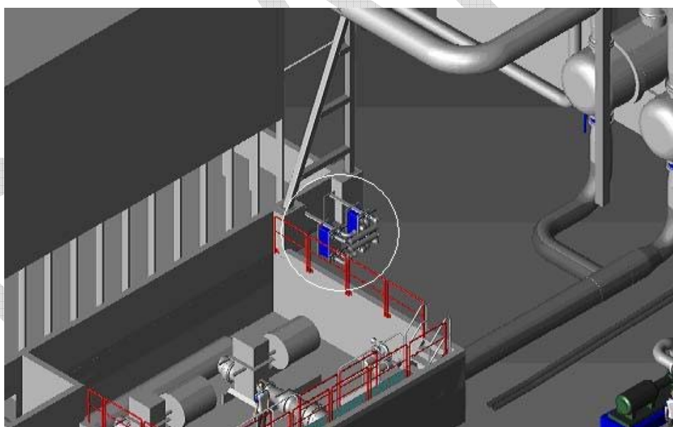
Figure 20: Auxiliary cooling loop heat exchangers.
