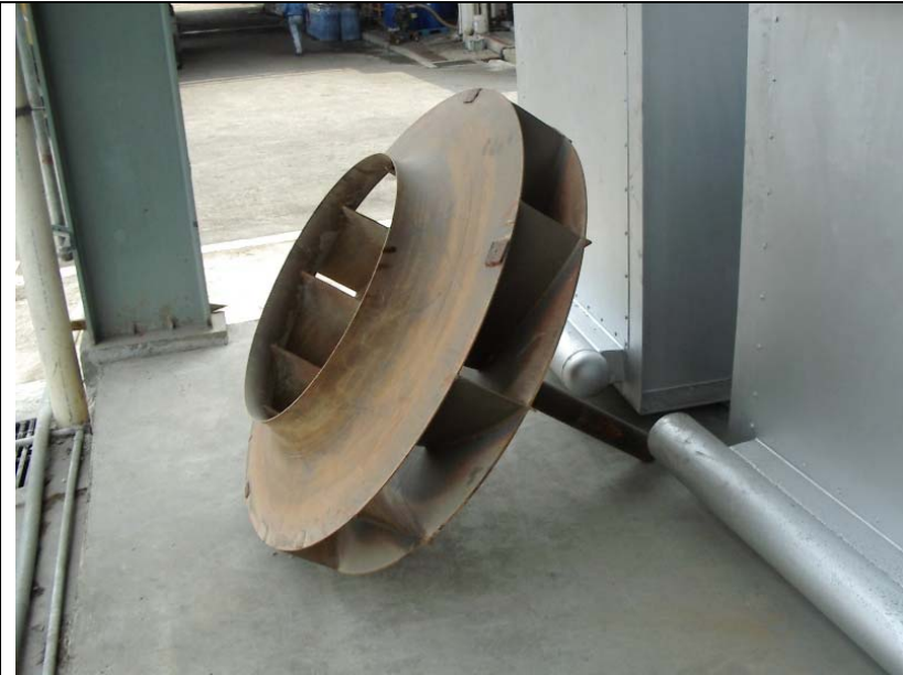
Figure 13: Damaged impeller of flue gas fan
