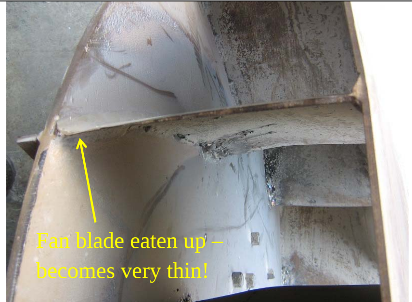
Figure 14: Impeller becomes paper thin due to excessive wear and tear
