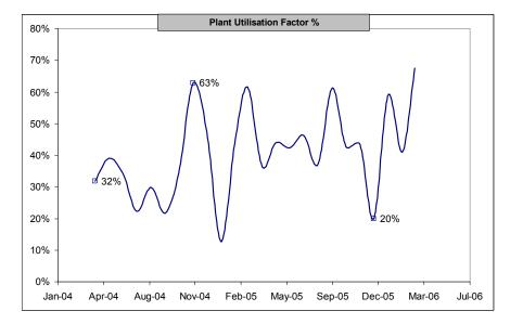
Low capacity utilization of kilns may be linked to operational problems, technological issues and unavailability of raw material for kiln operation. These reasons have been discussed in following section.
