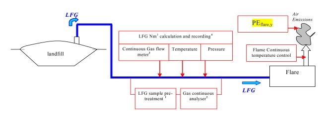
This monitoring methodology provides for direct and continuous measurement of the actual quantity of landfill gas fed to the flared and of the methane content of the landfill gas flared using a continuous flow meter and a continuous methane analyser. The continuous methane analyser is important because the methane content of landfill gas captured can vary by more than 20% during a single day due to gas capture network conditions (dilution with air at wellheads, leakage on pipes, etc.).
