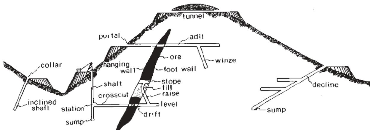
**Development** in an underground mine refers the creation of tunnels and other access routes that will allow the miner to access the ore. Development ends include areas such as:
