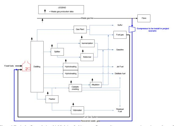
Figure 1 Typical refinery design, highlighting fuel inputs, refinery and waste gas generation points and use of recovered waste gas under the project activity
