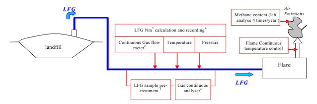
This monitoring methodology provides for direct and continuous measurement of the actual quantity of landfill gas flared and of the methane content of the landfill gas flared using a continuous flow meter and a continuous methane analyser. The continuous methane analyser is important because the methane content of landfill gas captured can vary by more than 20% during a single day due to gas capture network conditions (dilution with air at wellheads, leakage on pipes, etc.).
