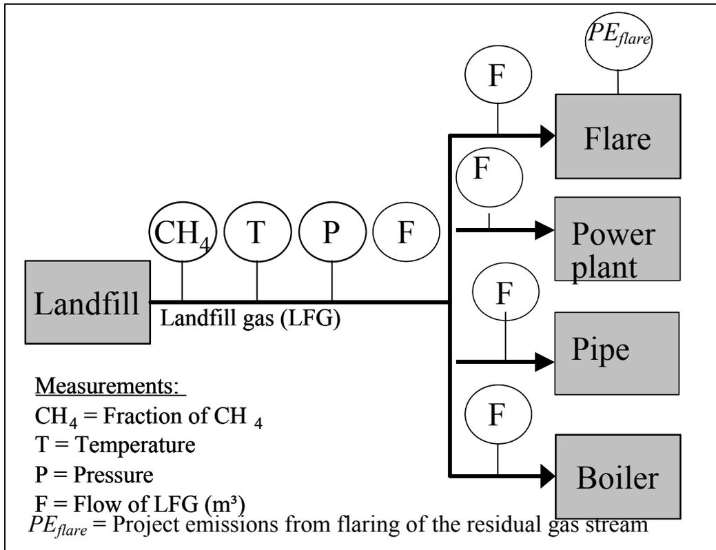
To determine these variables, the following parameters have to be monitored:
