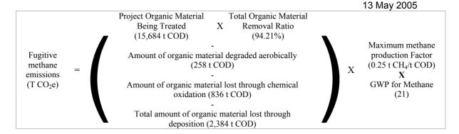
Fugitive methane emissions (t CO<sub>2</sub>e)  $= 59.304t \text{ CO}_2e$
