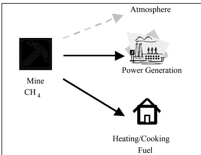
For eligible project activities, some or all of the MM/VAM used to generate electricity would be emitted to the atmosphere under the baseline (Figure 1). Appropriate MM/VAM flow and concentration meters should directly measure the amount of methane delivered to the project electric generator.
