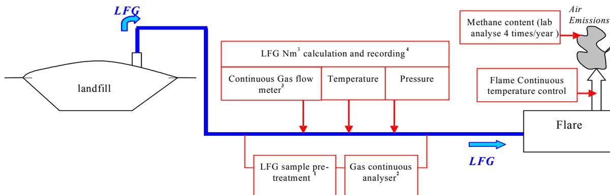
This monitoring methodology provides for direct and continuous measurement of the actual quantity of landfill gas flared and of the methane content of the landfill gas flared using a continuous flow meter and a continuous methane analyser. The continuous methane analyser is important because the methane content of landfill gas captured can vary by more than 20% during a single day due to gas capture network conditions (dilution with air at wellheads, leakage on pipes, etc.).
