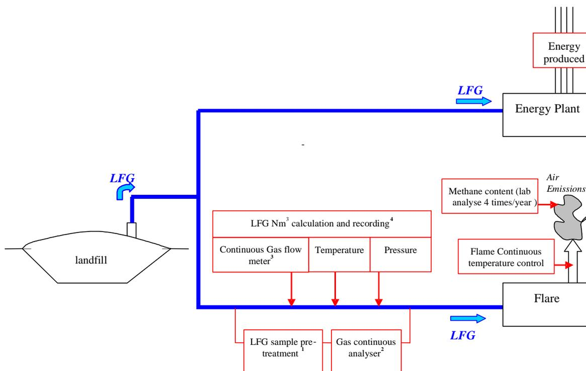
methane content of landfill gas captured can vary by more than 20% during a single day due to gas capture network conditions (dilution with air at wellheads, leakage on pipes, etc.).
